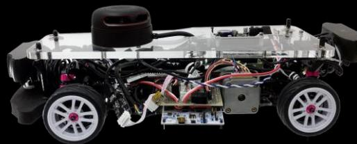
2D LIDAR RC Robot
